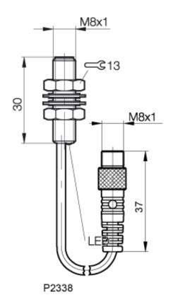
Inductive Sensors BES 516-371-E4-C-S49-00,3 D6.5 x 30 normally-open Sn=1,5mm shielded
